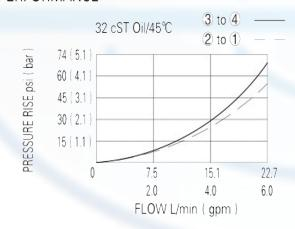
When de-energized, the valve allows flow from 3 to 4 and from 2 to 1; when energized, the cartrige's spool shifts to block flow at all ports.
