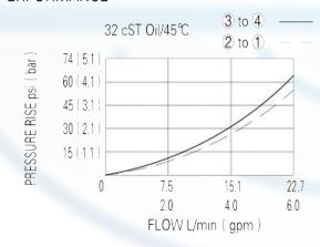
When de-energized, the valve allows flow from 2 to 1 and from 3 to 4; when energized, the cartrige's spool shifts and allows flow from 3 to 1, and is blocked at 2 and 4.
