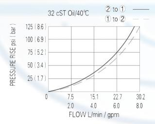
When de-energized, the valve blocks flow in both directionals, when energized, allowing flow from 2 to 1 and 1 to 2
