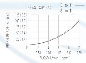
When de-energized, the valve allows flow from 3 to 1, while blocking flow at 2; when energized, the valve allows flow from 2 to 1, while blocking flow at 3.
