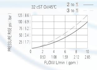
When de-energized, the valve allows flow from 2 to 1, while blocking flow at 3; when energized, the valve allows flow from 3 to 1, while blocking flow at 2
