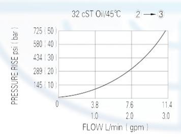
In its steady state, the valve blocks flow at 1, while allowing flow to pass from 2 to 3. On attainment of a pre-determined presssure at 1, the cartridge shifts to open at 1 to 2.
