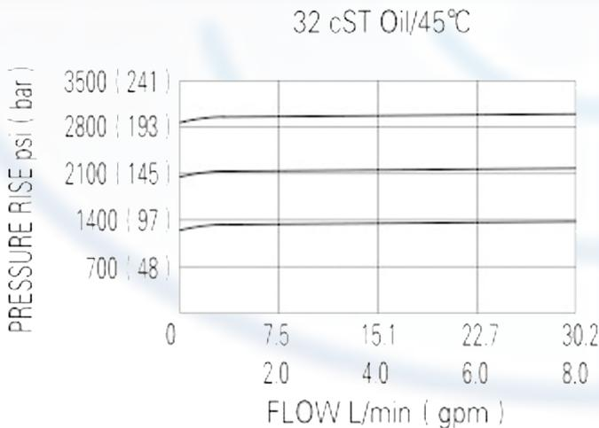
The valve prevents flow from 1 to 2 until the set crack pressure at 1 is achieved.
