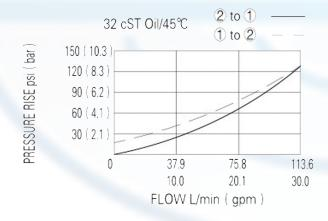
When de-energized, the valve acts as a check valve, allowing flow from 1 to 2, while blocking flow from 2 to 1;
