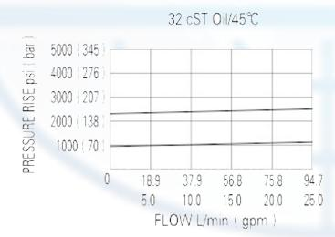
The valve prevents flow from 1 to 2 until pressur at 1 exceeds the set crack pressure and open the pilot section.
