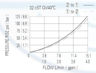
When de-energized, the valve blocks flow in both directionals, when energized, allowing flow from 2 to 1 and 1 to 2
