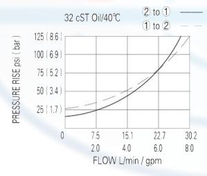
When de-energized, the valve acts as a check valve, allowing flow from 1 to 2, while blocking flow from 2 to 1;
