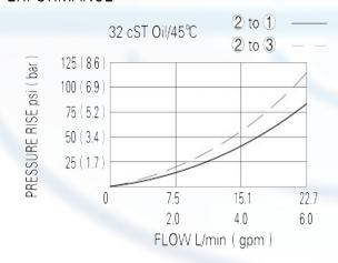
When de-energized, the valve allows flow from 2 to 1, while blocking flow at 3; when energized, the valve allows flow from 2 to 3, while blocking flow at 1.
