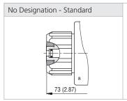
In case of solenoid malfunction or power failure, the spool of the valve can be shifted by manual override as long as the pressure in port T does not exceed 25 bar (363 PSI).
